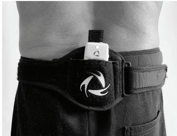
Fig. 1. The assessment of temporo-spatial variables during gait using an inertial sensors
