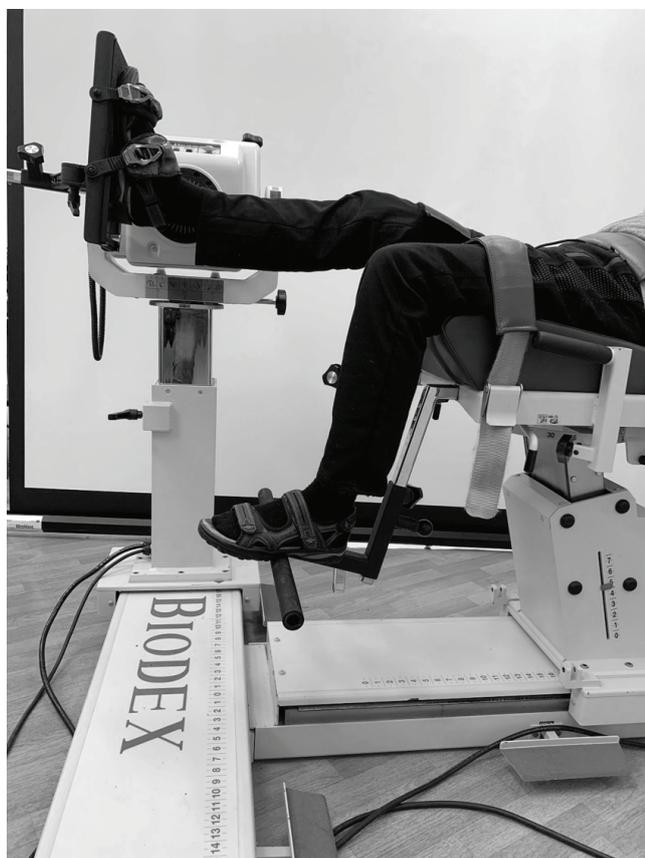
Fig. 2. The assessment of power-velocity capabilities of lower limb using a dynamometer
