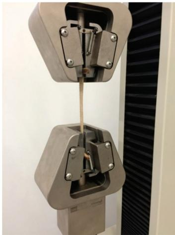
Fig. 1. A method of fixation of a sample in the clamps of the strength testing machine
