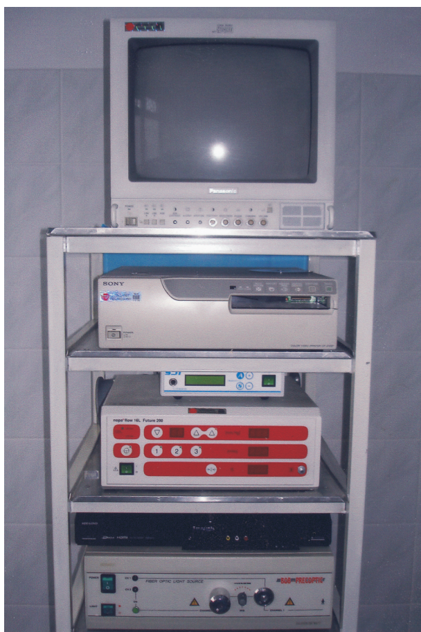
Fig. 1. Laparoscopic unit. From top to bottom: monitor, printer, camera, insufflator, DVD recorder, source of light.
