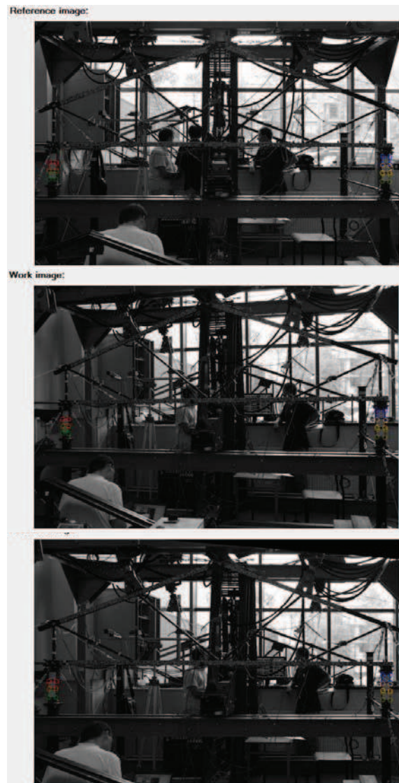
Fig. 1. Homography transformation: the reference image, the image with perspective distortion ( taken by the second camera), the second image after rectification
