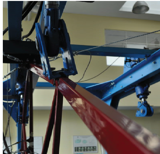
Fig. 13. Deformed truss in the point of jack mounting
