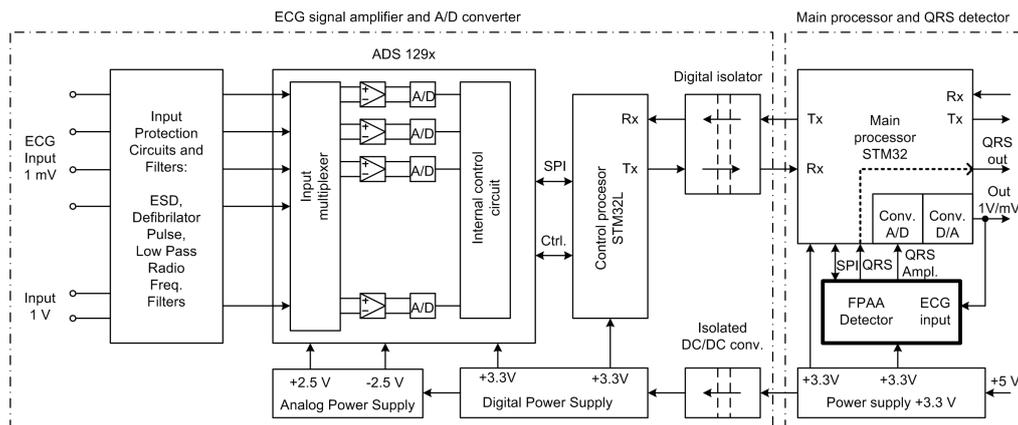
Fig. 1. The Block diagram of the ECG amplifier and QRS detector for VAD.
