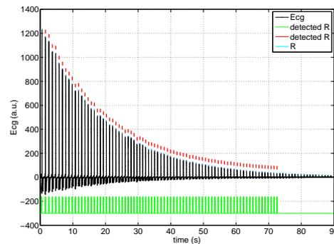
Fig. 7. An example of QRS detection without re-configuration of the ADS129x, the acceptable range of amplitude changes 1:36.
