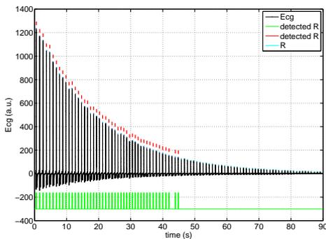
Fig. 6. An example of QRS detection without AGC (with constant parameters), the acceptable range of amplitude changes 1:8.
