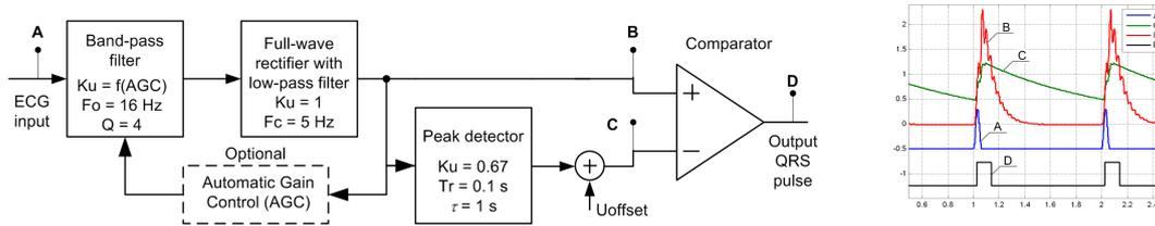
Fig. 2. The block diagram of the analog QRS detector (left) and simulation results (right).
