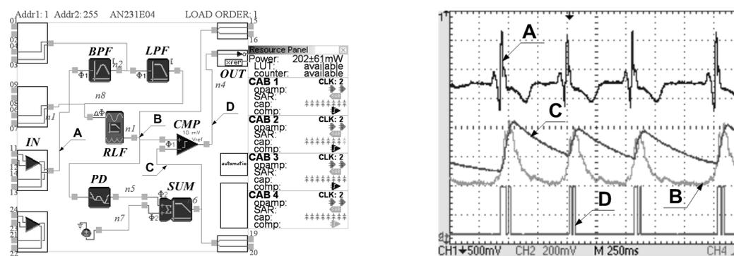
Fig. 3. The QRS detector implementation in the FPAA (left) and waveforms in the characteristic nodes (right).
