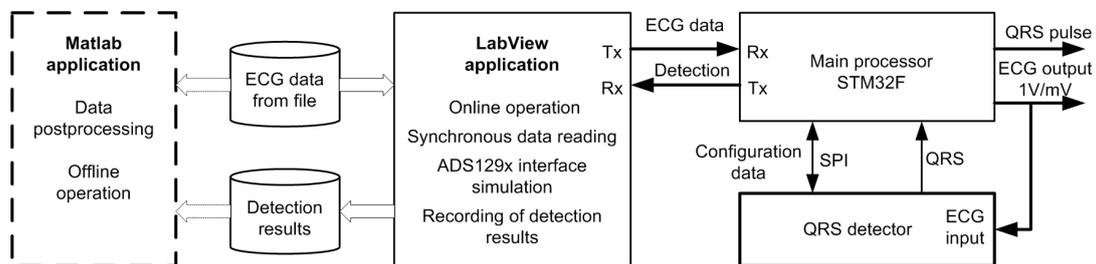
Fig. 4. The block diagram of test procedures.
