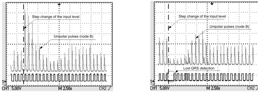
Fig. 5. The system response to a step 3-fold increase in amplitude (left) and step 5-fold decrease in the amplitude (right).
