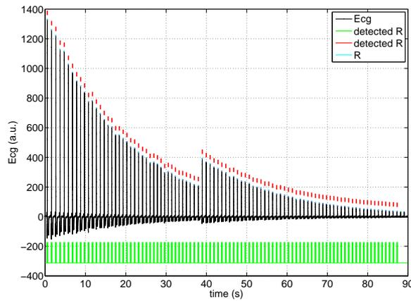
Fig. 8. An example of QRS detection with AGC and reconfiguration of the ADS129x, the acceptable range of amplitude changes 1:72.
