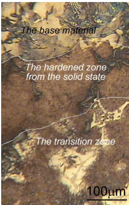
Fig. 7. The microstructure of the cross section through the transition zone, hardened zone from the solid state to core material in the surface layer of malleable iron after laser heat treatment. Etched with nitride acid solution
