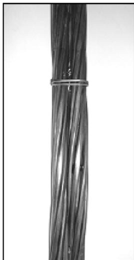
**Fig. 3.** Double “nutcage” rope tendon [8]
