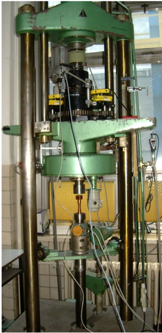
Fig. 1. Universal machine for testing materials under complex loading conditions
