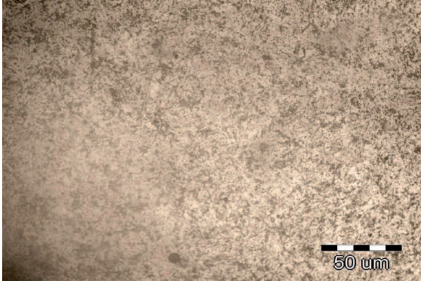
Fig. 7. Microstructure of steel hardened and tempered at 500°C. Sorbit – mixture of ferrite and submicroscopic carbides. Hardness 316 HV. Mag. 500x
