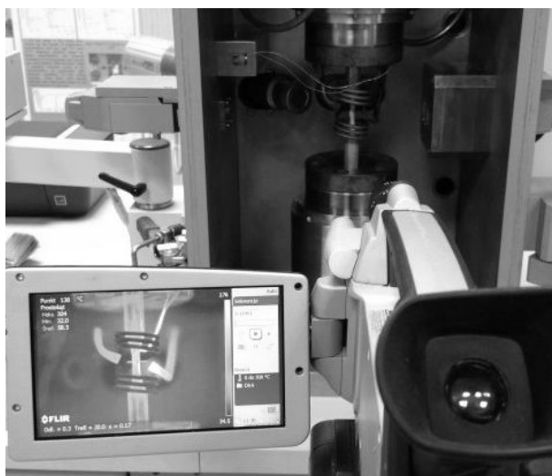
Fig. 2. Temperature measurement of the sample using thermovision technology
