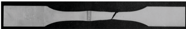
Fig. 13. A view of the broken sample from the tensile tests of the butt joint A(3) welded at 1.6 kW and welding speed of 0.2 m/min (heat input of 480 J/mm, Tab. 4)
