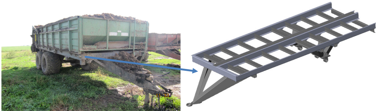
Fig. 1. Trailer – spreader of type RTD: general view of the bearing system
