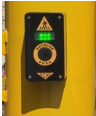
Fig. 1. Button of a traffic light for alerting the system a pedestrian is waiting
