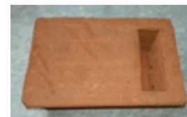
Fig. 5. A sand mould with an oil binder, OBB Sand
