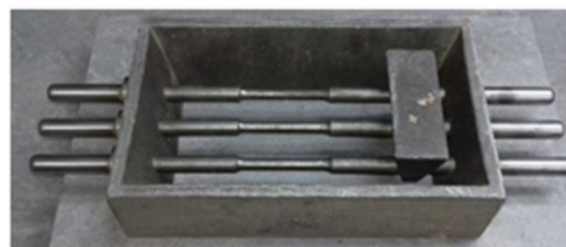
Fig. 3. The set-up for making sand moulds
