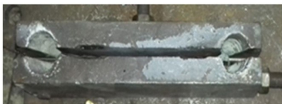
Fig. 6. A divided metal mould
