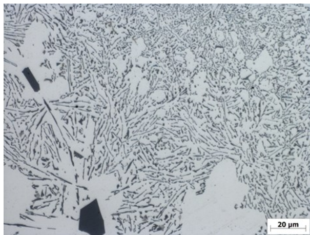
Fig. 6. Microstructure of samples, pressure 150 MPa, temperature 715°C, etched with 0.5% HF
