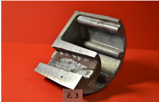
Fig. 7. Test with the VŠB – TUO glue during dissolution of the glued core
