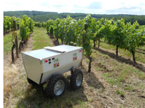
Fig. 8. Car-like Vine robot [17]
