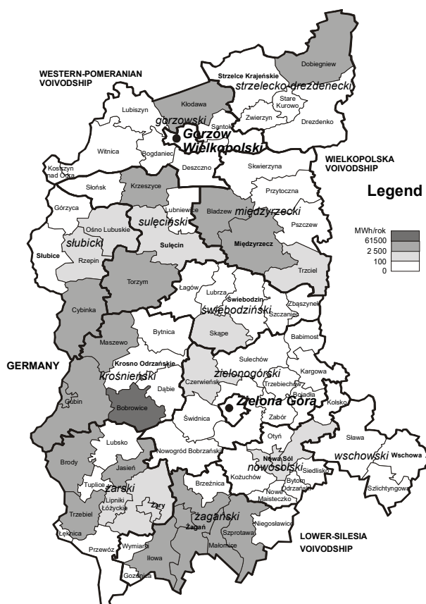
Fig. 17. The water energy potential possible to achieve with the existing dams [MWh/year] (Source: prepared by the author, based on [16])
