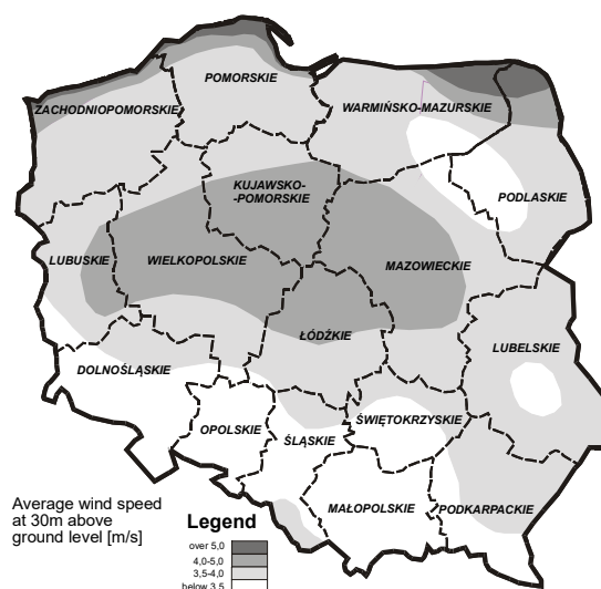
Fig. 6. A map of wind speed zones at 30 m above ground level. [m/s] (Source: prepared by the author, based on [18])
