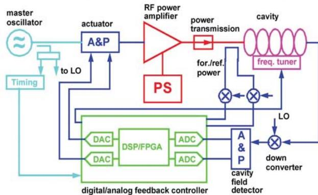
Figure 1. LLRF System Architecture
