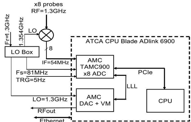
Figure 2. Hardware block diagram for the first demonstration
