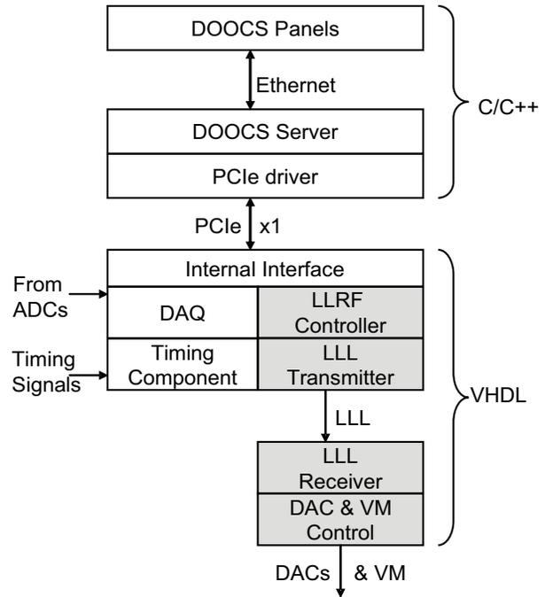
Figure 6. Architecture of software used in tests
