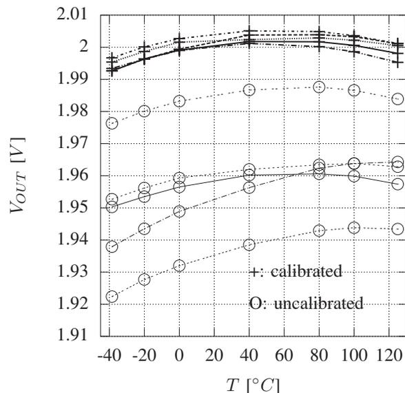
Fig. 20. Measurement of five different typical chips: Comparison between uncalibrated and calibrated output voltages at  $V_{DD} = 3.3V$  and  $T = 25^\circ C$ . Both temperature coefficient and offset were compensated.
