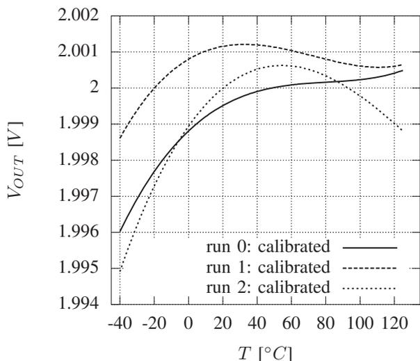
Fig. 14. Detailed view of the three examples for offset and tempco calibration (calibrated curves only)
