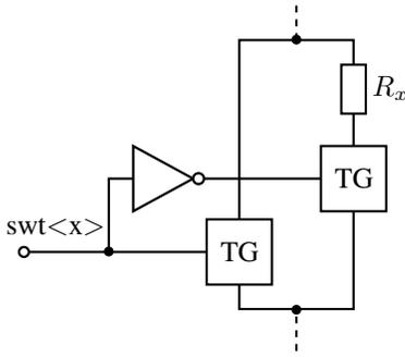
Fig. 6. Block diagram of a single resistor element of  $R_{swt}$
