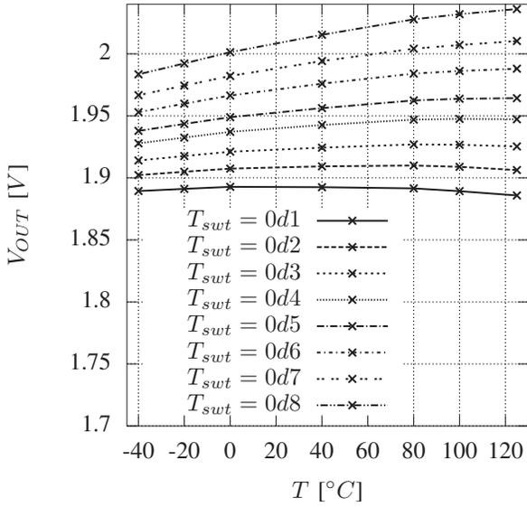
Fig. 16. Measurement of the trimmable temperature coefficient of the overall circuit (with untrimmed offset)
