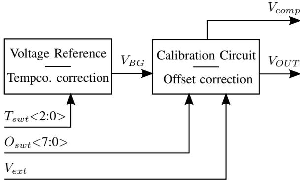
Fig. 2. Block diagram of the trimmable voltage reference
