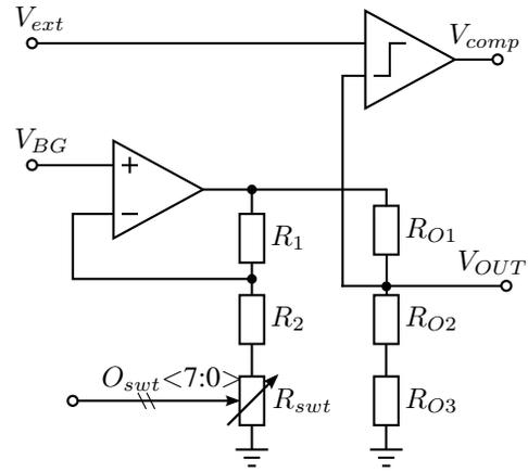
Fig. 7. Schematic of the offset calibration circuit
