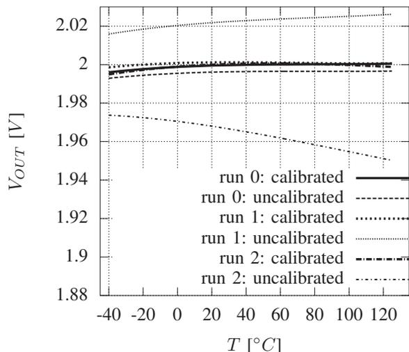
Fig. 13. Three simulation examples for offset and tempco calibration (uncalibrated curves are slashed, calibrated curves solid)
