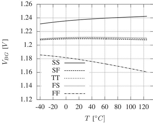
Fig. 8. Change of the temperature coefficient of TBGR due to process variations
