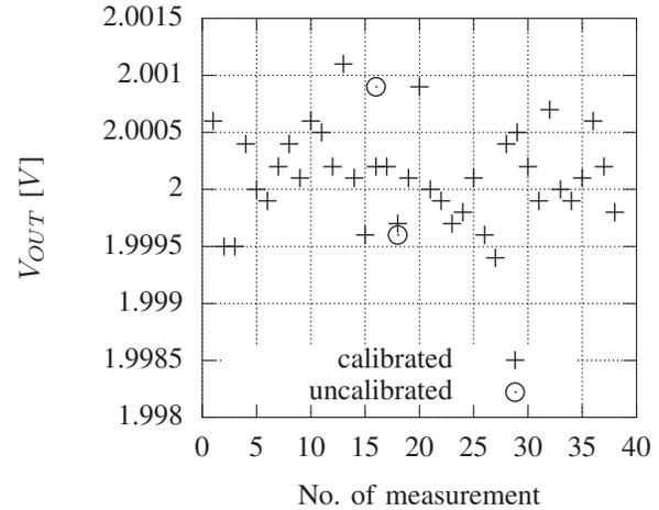
Fig. 19. Measurement of 38 different corner chips: Comparison between uncalibrated and optimally offset calibrated output voltages at  $V_{DD} = 3.3V$  and  $T = 25^{\circ}C$ .
