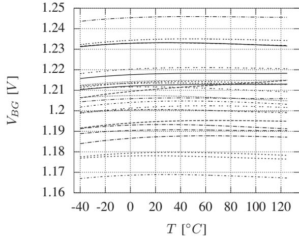
Fig. 10. Monte-Carlo analysis of a trimmed TBGR output voltage
