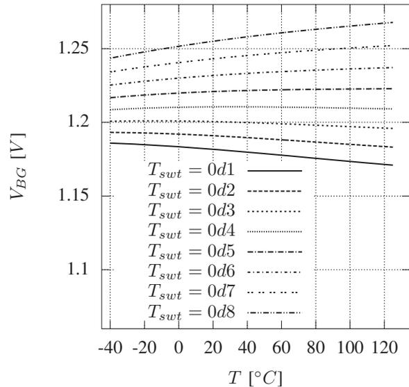
Fig. 5. Simulated range of the calibratable temperature coefficient of output voltage  $V_{BG}$  of the TBGR
