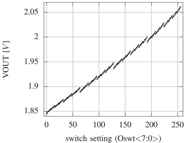
Fig. 17. Measurement of the offset calibration of the overall circuit (with untrimmed temperature coefficient)
