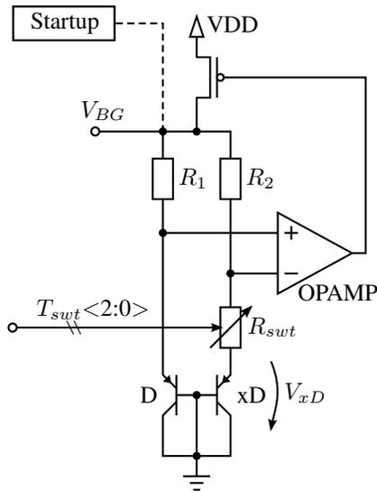
Fig. 3. Schematic of the trimmable bandgap reference
