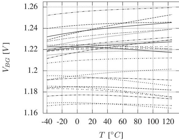
Fig. 9. Monte-Carlo analysis of an untrimmed TBGR output voltage
