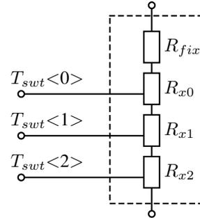
Fig. 4. Block diagram of  $R_{swt}$
