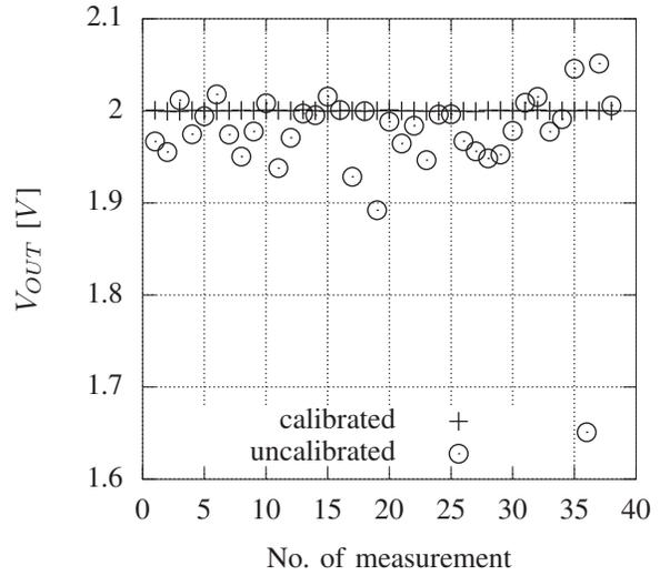
Fig. 18. Measurement of 38 different corner chips: Comparison between uncalibrated and optimally offset calibrated output voltages at  $V_{DD} = 3.3V$  and  $T = 25^{\circ}C$ .
