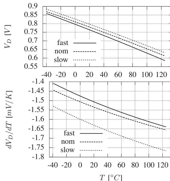
Fig. 1. Temperature characteristics of the diode-connected BJT due to process variations
