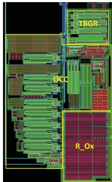
Fig. 15. Layout of the proposed voltage reference
