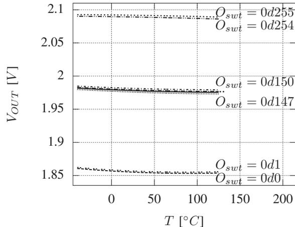
Fig. 12. Simulated offset calibration range ( $O_{swt}=0$  (min),  $O_{swt}=255$  (max) and some sample values in between ( $O_{swt}=1, 147, 148, 149, 150, 254$ ))
