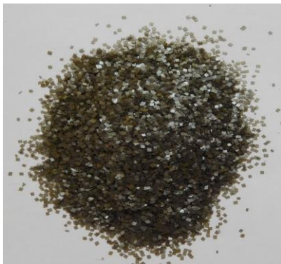
Fig. 3 (a). Double base propellant
