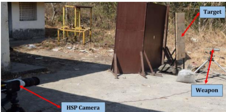
Fig. 4. An experimental set-up for measurement of velocity of water-jet using a high-speed camera. It consists of camera, water-jet disruptor and target for arresting the projectile using the firing stand
