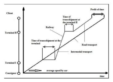
Fig. 3. Comparison of the time of road transport and railway-road transport
