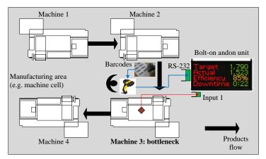
Fig. 2 A scheme of bolt-on andon installation in manufacturing area
