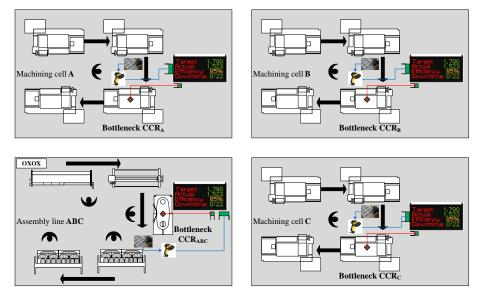
Fig. 3 Practical example: the scheme of mini factory for KPIs calculation
