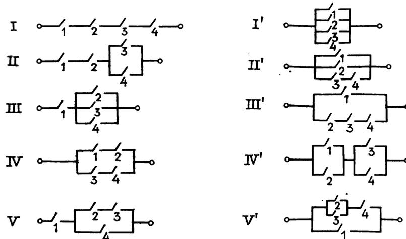
Fig. 1. Two-terminal series-parallel structures built of 4 components
