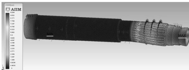
Fig. 5. Fields of the displacement of spindle
