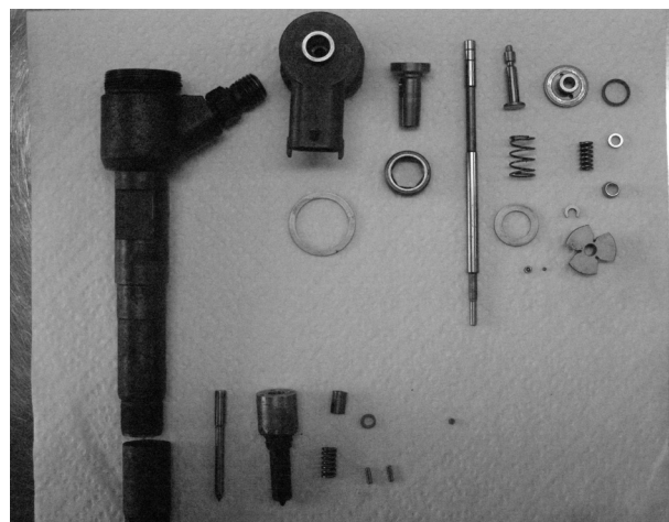
Fig. 2. Electromagnetic Bosch generation 1.0 injector disassembled into spare parts
