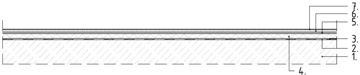
**Fig. 7** Point-elastic floor without a grid with synthetic poured surface
