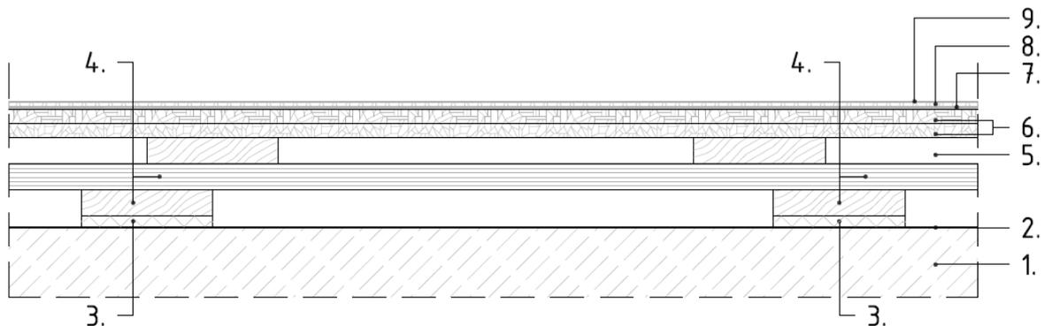
**Fig. 4** Area-elastic floor on a grid with synthetic poured surface
