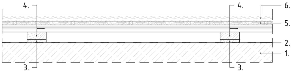
**Fig. 2** Area-elastic floor on a grid with wooden surface
