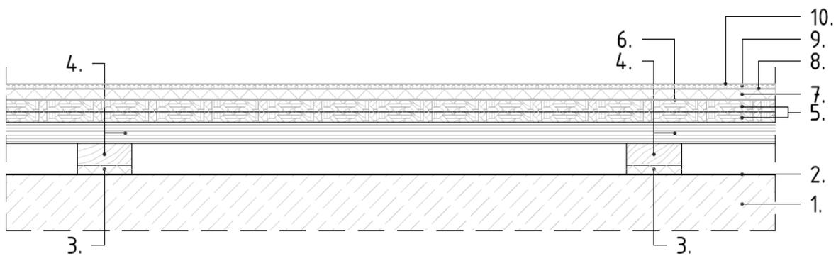
**Fig. 3** Combined-elastic floor on a grid with synthetic poured surface
