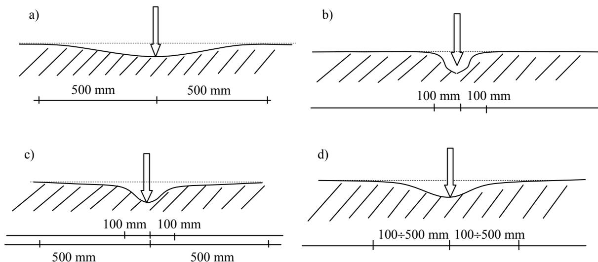
**Fig. 1** Sports floor behaviour scheme under load
