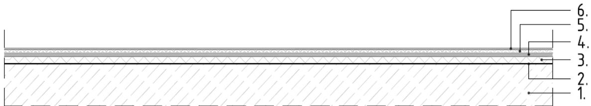
**Fig. 6** Area-elastic floor without a grid with synthetic rolled surface
