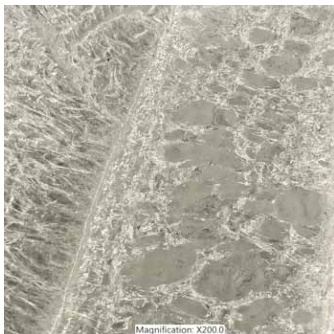
Fig. 3. Pictures of microporous polypropylene Acurell® XP 100-84 obtained by: a) digital microscope Keyence VHX 6000, 200\times magnification, b) micro-computed tomograph SkyScan 1272 by Bruker; picture presents cross-section (approximately 2.6 mm in diameter) of investigated sample with scanning resolution of 2 \mu\text{m}
