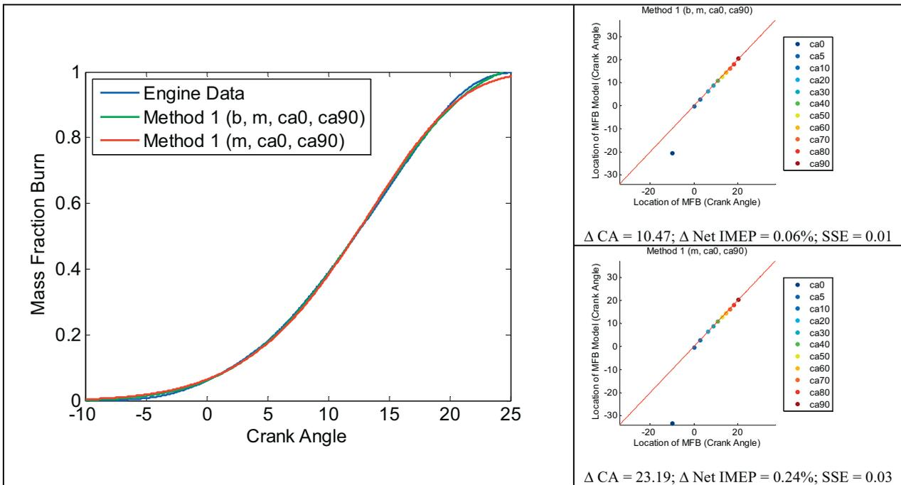
Fig. 1. The mass fraction burn and the Wiebe fitted curve using Method 1 (Gasoline, CR = 8.0:1, spark advanced = 10° BTDC, speed = 900 RPM, load = 330 kPa Net IMEP)
