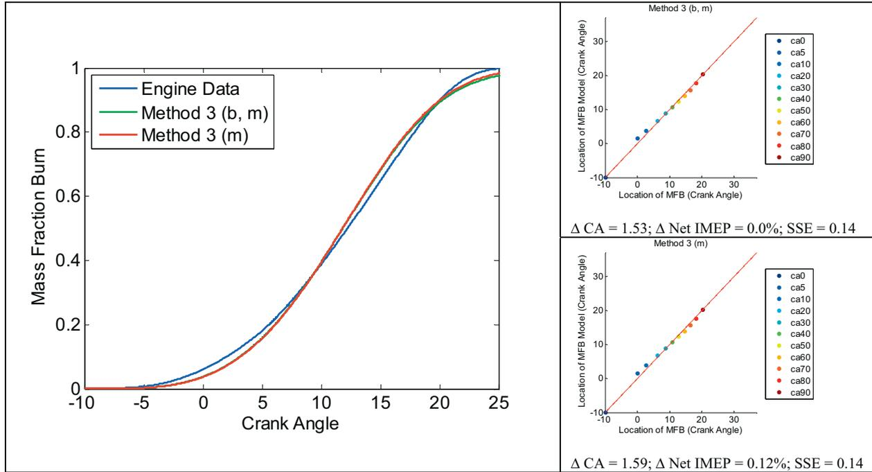
Fig. 3. The mass fraction burn and the Wiebe fitted curve using the method 3 (Gasoline, CR = 8.0:1, spark advanced = 10° BTDC, speed = 900 RPM, load = 330 kPa Net IMEP).
