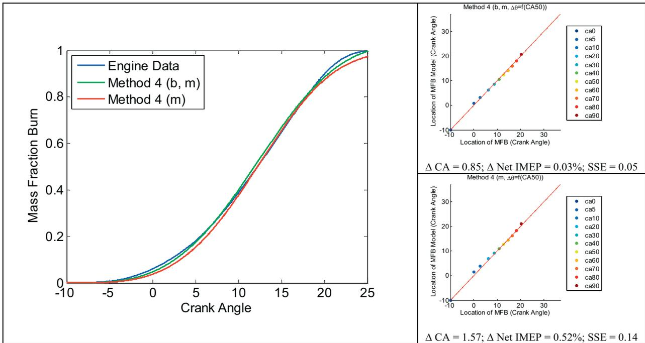
Fig. 4. The mass fraction burn and the Wiebe fitted curve using the method 4 (Gasoline, CR = 8.0:1, spark advanced = 10° BTDC, speed = 900 RPM, load = 330 kPa Net IMEP).
