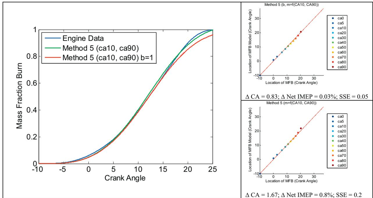
Fig. 5. The mass fraction burn and the Wiebe fitted curve using the method 5 (Gasoline, CR = 8.0:1, spark advanced = 10° BTDC, speed = 900 RPM, load = 330 kPa Net IMEP)
