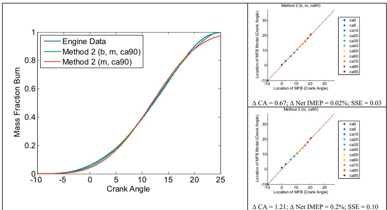
Fig. 2. The mass fraction burn and the Wiebe fitted curve using the Method 2 (Gasoline, CR = 8.0:1, spark advanced = 10° BTDC, speed = 900 RPM, load = 330 kPa Net IMEP)
