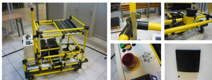
*Fig. 1. The AGV modular construction type*
