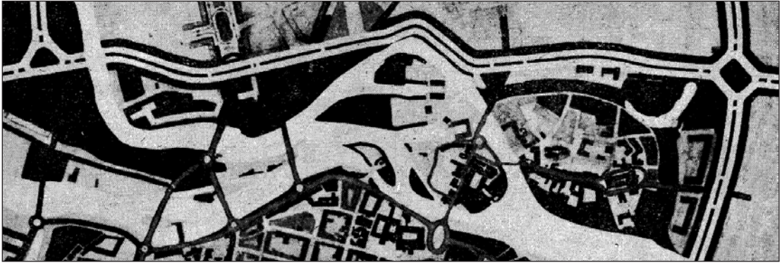
46. Fragment of the spatial development plan of Wrocław from 1949, developed by a team led by Emil Kalliski. The communication route connecting the small and large central city beltway was passed through the Sand Island. In order to preserve the historical character of the remaining buildings, traffic from the city center was divided into two directions served by Staromłyńska Street (at the back of the island) and Piaskowa Street. Both streets were to be connected through a newly designed roundabout at the Mill Bridge. There were no plans to restore the buildings on the islands of Słodowa and Bielarska (except for St Clare's Mills and the surviving residential building on Słodowa Island) – these areas were designated for sports facilities and greenery. The buildings of Kępa Mieszcząńska were to be preserved. It was planned to reconstruct the north frontage of Katedralna street, including historical building lines [92, p. 125]
