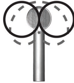
Fig. 106. MS microphone positioning – top view.
