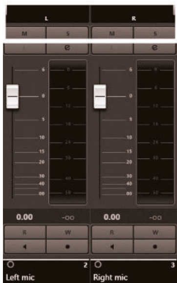
Fig. 104. Proper microphone panning used in the Blumlein technique (marked with the white rectangle).
