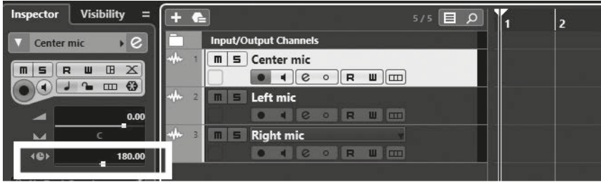
Fig. 99. An alternative microphone panning used in the X-Y + M technique (marked with the white rectangle). The central microphone track has a digital signal delay of 180 ms to eliminate phase issues of sounds reaching the central microphone. Consequently, the delay line is unnecessary as the delay is ensured differently.
