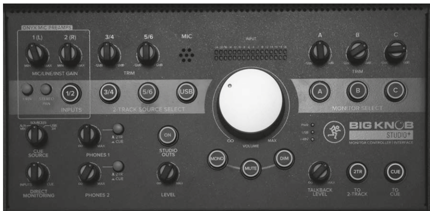
Fig. 51. Monitor controller for various studio monitors (front panel).
