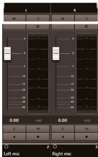
Fig. 101. Proper microphone panning used in the ORTF / NOS technique (marked with the white rectangle).
