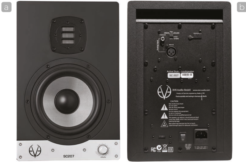
Fig. 44. a) and b) Front and back of an active near-field studio monitor with a bass reflex port in the form of a long and narrow rectangular vent, mounted at the back. One of the sides for low-frequency propagation is wider and semi-circular in shape.
