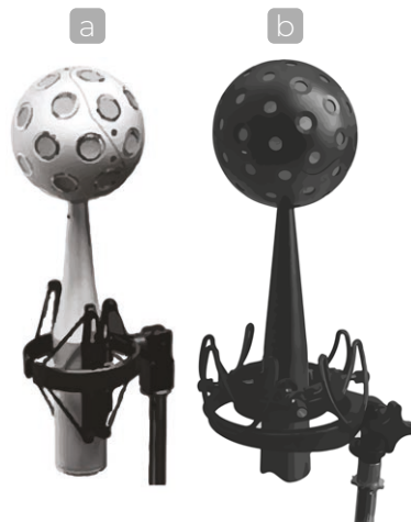
Fig. 27. a) 32-channel surround microphone and b) 64-channel surround microphone.
