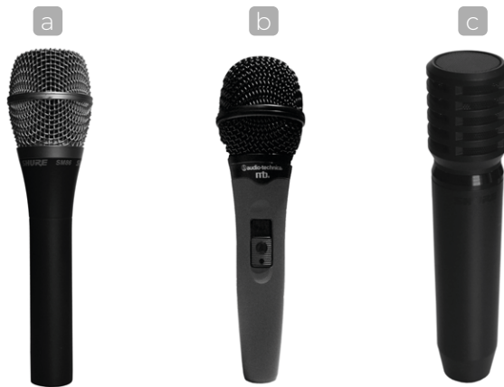
Fig. 3. a) – c) A selection of dynamic microphones used onstage by the vocalists. Each device comes equipped with a uniquely shaped head which covers the diaphragm converting the acoustic signal to the electric signal.
