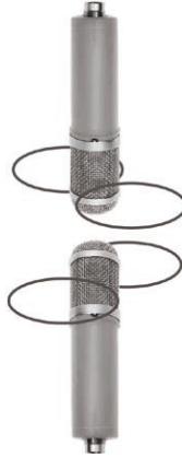
Fig. 102. The layout of microphones in the Blumlein technique.
