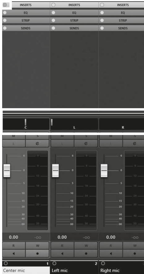
Fig. 98. Proper microphone panning used in the X-Y + M technique (marked with the white rectangle). A special delay line was used for the inserts to avoid the phase difference of the sounds reaching the central microphone.
