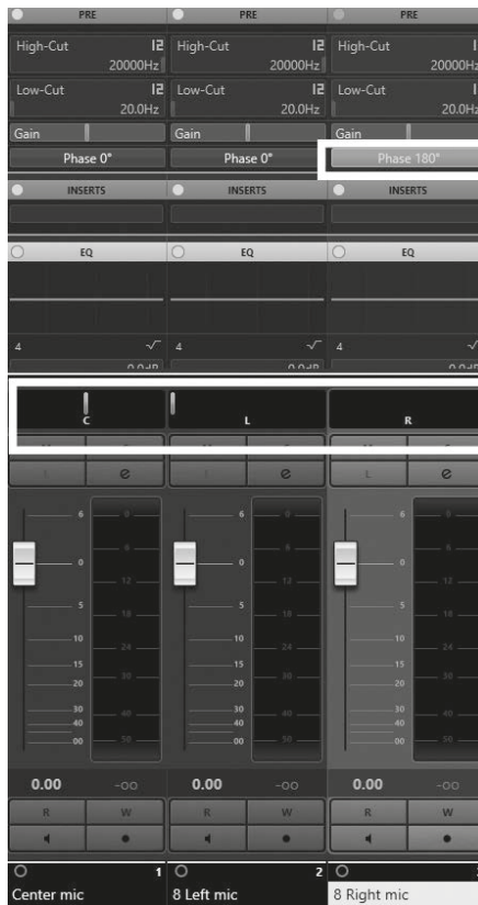
Fig. 107. Proper microphone panning used in the MS method including the necessary phase reversal by 180 degrees in one of the channels (marked with the white rectangle).
