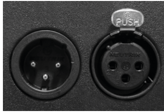
Fig. 72. Male (to the left) and female (to the right) XLR sockets mounted in an electronic device.
