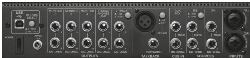
Fig. 52. Monitor controller for various studio monitors (rear panel).
