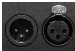
Fig. 78. Digital AES / EBU sockets (identical to XLR on the outside).
