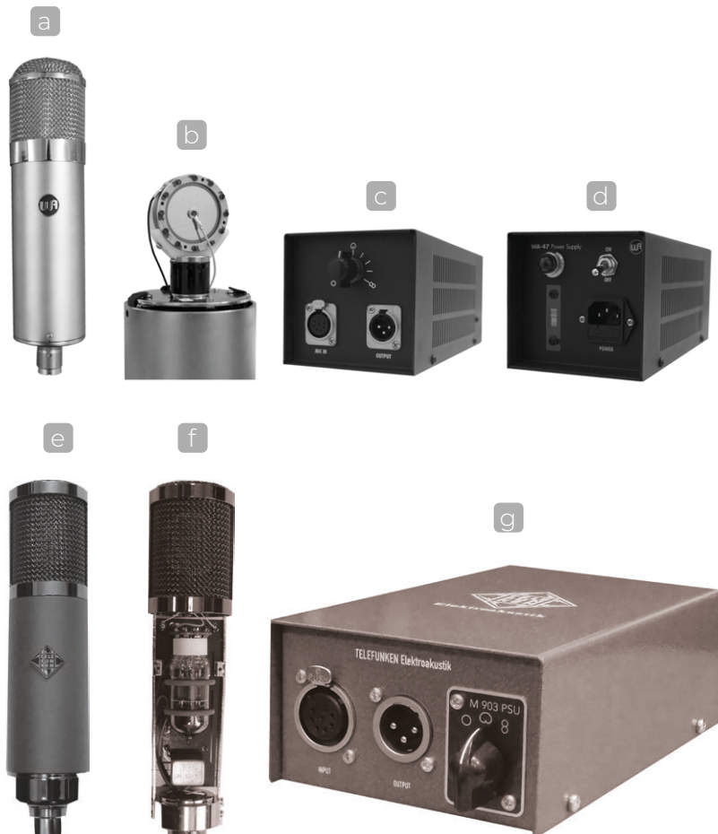
Fig. 12. a) – g) Tube microphones feature a tube which imbues the processed sound with the characteristic warm tonality as even harmonics are added to the audio signal. Tube microphones always come with a specialized cable for the power supply unit, which transmits both audio and the electrical current. The power supply generates electricity to power the tube correctly and allows for power modulation, which produces various directionality characteristics. The sockets are usually constructed to prevent a direct connection to the mixing console with an XLR connector since phantom power could damage the device. A tube microphone connected to the mixing console through the supply unit can operate without phantom power, as the device sends a correct sound signal which does not need an additional power supply.
