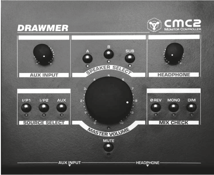
Fig. 53. Monitor controller for various studio monitors (front panel).
