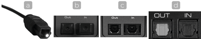
Fig. 77. a – d) Toslink fibre-optic connector (top-left corner) with sockets closed with protective anti-dust caps (centre of the upper row), sockets open with the caps off (top-right corner), and sockets with an automatic anti-dust block (centre of the lower row).
