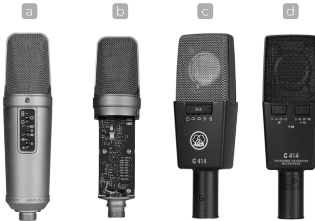
Fig. 8. a) – d) Large-diaphragm condenser microphones exhibiting multi-directionality (their sound pickup patterns can be switched by the user) are deployed in recording studios. They operate properly on phantom power, supplied from such sources as the recording device or a mixing console. The multi-pattern directionality allows for optimally positioning the microphone relative to the source of sound propagation so that the device captures the audio from the selected space fragment only while suppressing other (unwanted) sounds. Additionally, such microphones often come equipped with a signal attenuator labelled as “pad” (several to twenty dB) and can cut off selected low frequencies to eliminate thumping during the recording process.
