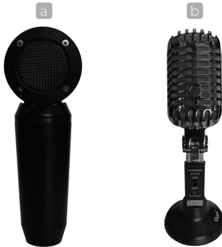
Fig. 5. a) and b) The figure presents dynamic microphones often used by the vocalists. Their structure differs from traditional dynamic microphones as the diaphragm remains in the vertical position or at an angle.
