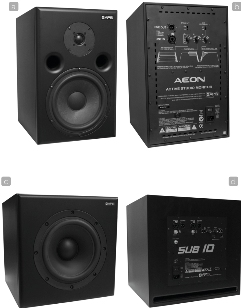
Fig. 48. a) – d) Front and back of an active near- and mid-field studio monitor with two circular bass reflex vents at the front together with a subwoofer for processing low frequencies. In this case, the subwoofer expands the range of the low frequencies processed, complementing primary drivers. Its bass reflex port is a long and narrow rectangular vent with rounded sides, mounted at the back.
