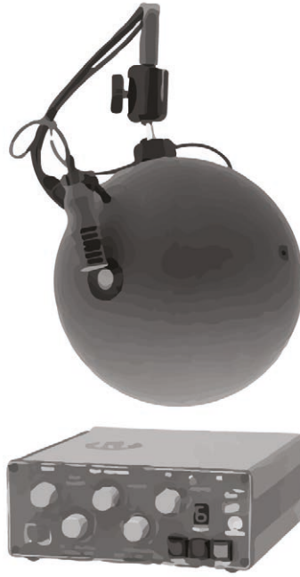
Fig. 22. A multichannel microphone (dummy head) made of special material. Since the microphones are placed to mirror the location of human ears, the device can simulate binaural hearing.
