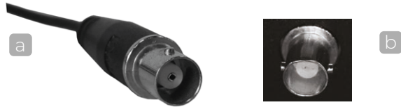
Fig. 82. a) and b) Coaxial MADI sockets on the cable (to the left) and installed in an electronic device (to the right).
