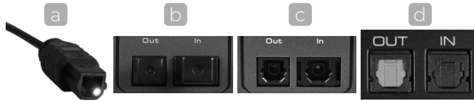
Fig. 80. a) – d) ADAT plug and sockets (identical to Toslink on the outside).
