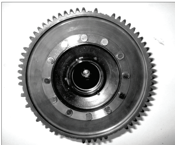
Fig. 3.53. Damaged gear wheel in the gearbox of a Mi-24 helicopter
