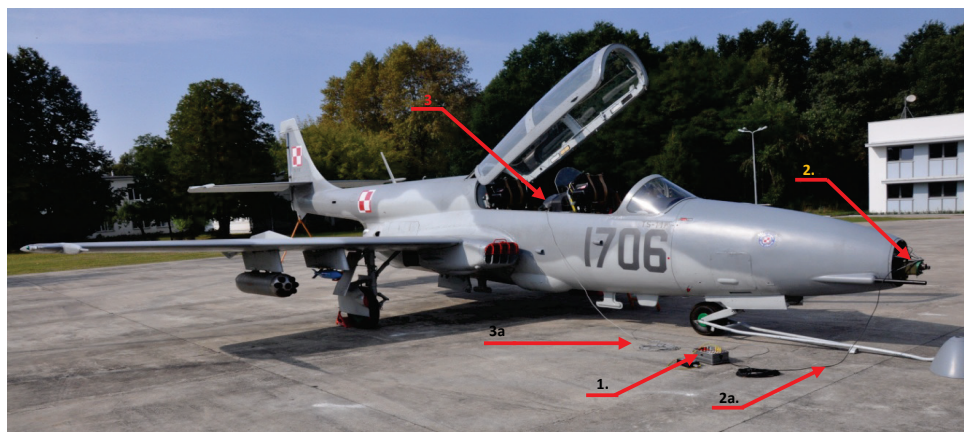
Fig. 5.13. TS-11 Iskra aircraft with a connected DIA-SO3 diagnostic tester: 1 – diagnostic tester DIA-SO3, 2 – 28V DC socket (nose cone part of the fuselage) – tie-in location for a DC measurement channel of the DIA-SO3 tester circuit, 2a – electrical cable connecting the 28V socket and the tester, 3 – tachometer connector (dashboard in the second cabin) – tie-in location of the AC measurement channel (three-phase) to the DIA-SO3 tester, 3a – electrical cable connecting the tachometer connector with the tester
