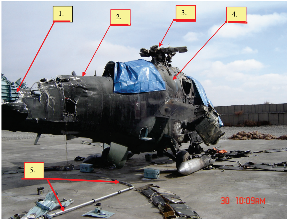
Fig. 5.24. Mi-24 helicopter with a transmission system discontinued due to internal damage in the generator gearbox: 1 – place of the torn-out generator gearbox, 2 – sheathing over a surviving transmission segment, 3 – main rotor hub after blade disconnection, 4 – WR-24 main transmission cover (movable), 5 – auxiliary rotor propulsion transmission torn out and bent as a result of the helicopter hitting the ground
