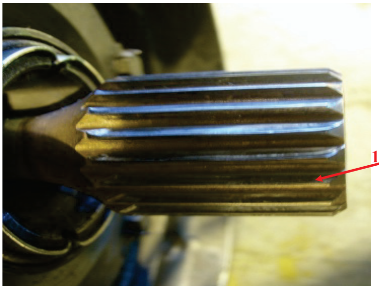
Fig. 3.16. Splined shaft of a GT-40PCz6 AC generator under long-term operation with skew and eccentric displacement: 1 – trace of material loss on the drive shaft splines in the shape of “conical” decrements on the contact plane
