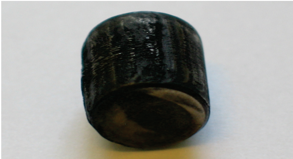
Fig. 3.39. Rolling element of a bearing with excessive clamp and traces of “milling” and surface rippling caused by excessive thermal energy release
